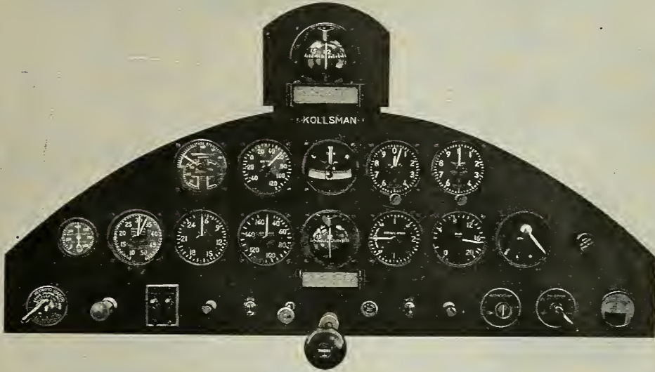
KOLLSMAN INSTALLATION OF CLAMP-TYPE INSTRUMENTS FLUSH FRONT MOUNTED AND INDIVIDUALLY LIGHTED
